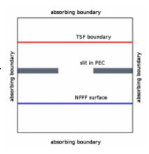
Near-to-far field transformation (NFFF) integrated from plane behind the aperture is used to calculate far field radiation pattern. Preserving both TSF source and NFFF integration plane close to metal plane helps to minimize influence of finite plane wave and metal plane size.
