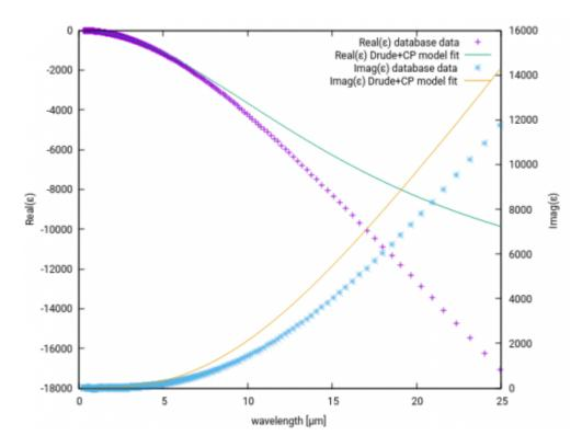
The solution is to fit a suitable dielectic function model to the database data and use this in the calculation. For metals in infrared a Drude model is typically recommended. This can be handled via the PLRC and ADE algorithm, for example by setting the strength of critical points to zero in any of the Drude+CP algorithms. The dielectric function fitted to a particular wavelength range, here around 10 microns, looks already much better:
