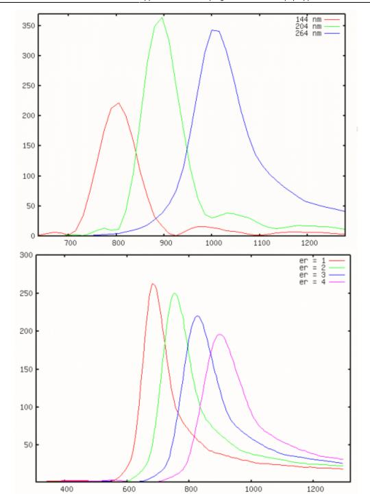
Similar results can be obtained for two triangular metallic objects used as nanoantenna (see the simulation snapshot in the right figure). Here a spectral dependence of the field enhancement between the objects is shown for two different sizes of the whole system (I: total length, g: gap width)
