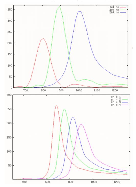
Similar results can be obtained for two triangular metallic objects used as nanoantenna (see the simulation snapshot in the right figure). Here a spectral dependence of the field enhancement between the objects is shown for two different sizes of the whole system (I: total length, g: gap width) for wavelengths from 300 to 1300 nm.
