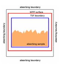
To evaluate far field scattering pattern, a NFFF computational boundary is established around computational volume, just few voxels apart the absorbing boundary conditions.
