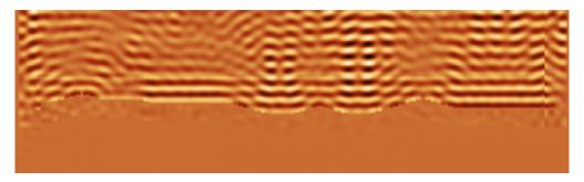
As a result we obtain a far field radiation pattern as shown below. We can see that roughness leads to scattering, which is obvious. The results can be directly compared to e.g. far field measurements using scatterometry when we have such measurement for particular surface. It is however necessary to perform simulation on statistically relevant surface, e.g. on surface large enough, or average multiple simulations on different images.
