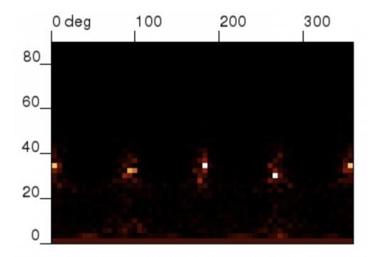
As we have simulated the surface, we know in advance what should be angular position of the maxima - they should be spaced by 90 degrees, with angle to normal of 32.5 degrees. Simulated data show the maximum at 33±2 degrees which is in agreement to this result; with better statistics the angle uncertainty should decrease furthermore.
