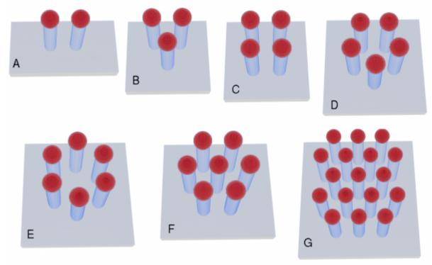
User can control the size of rod components, periodiciy and add some imperfections, like imperfection in the rod position and relaxation of the rod, as shown here.
