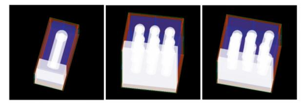
As an example of numerical results here we show resulting time averaged spatial distribution of absorption in single column structure illuminated from top (left) and bottom (right), for 500 nm illumination wavelength. Visualisation was performed using Paraview.
