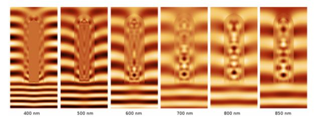
If we run full spectral calculation, we can get also dependences of summed local absorption in different parts of the solar cell, for distinct materials. A preliminary result for bottom illuminated regular structure is shown below (note that number of steps for longer wavelengths was too small for
