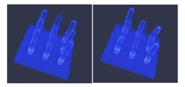
Geometrical model can be made even more complex, e.g. by adding scanning probe microscope tip to the structure. This geometry is similar to what we use in photoconductive AFM measurements. After adding simple tetrahedral tip we get this snapshot and volume absorption (tip only sketched on absorption image).
