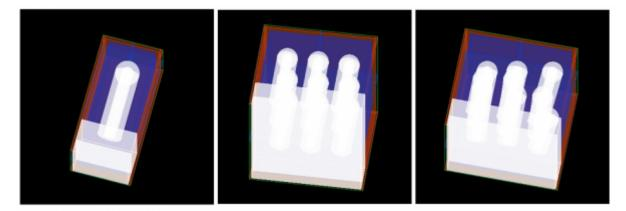
As an example of numerical results here we show resulting time averaged spatial distribution of absorption in single column structure illuminated from top (left) and bottom (right), for 500 nm illumination wavelength. Visualisation was performed using Paraview.
