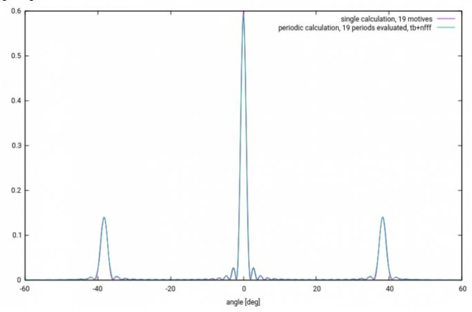
When inspected in detail, it can be seen that there is only a difference of about 0.2 percents between the two methods output for the first diffraction maximum, which was confirmed as a positive effect of bigger distance of the computed structure from boundaries. A bigger problem is, that the diffracted intensity is about 0.140 of the incident intensity, which is less than expected (the expected value is 0.186). Something has to be wrong.
